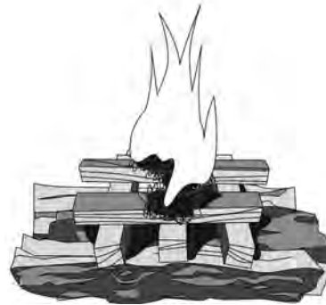
Fig. 4.7 | Combustible firelighter module on stack of fuelwood
