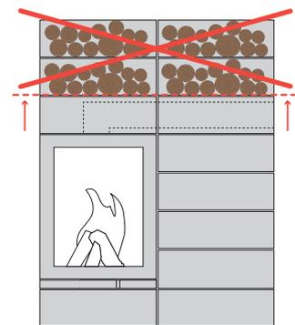
3. The storage of flammable materials above extension elements where smoke discharge tubes are fed through is not possible.
