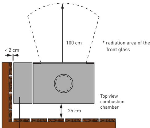
Extension element **without** smoke discharge tube
