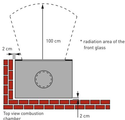
For »elements« with or without lateral extension elements, the above mentioned safety distance to **non combustible elements** and walls (such as concrete, stone, plaster) should be observed.
