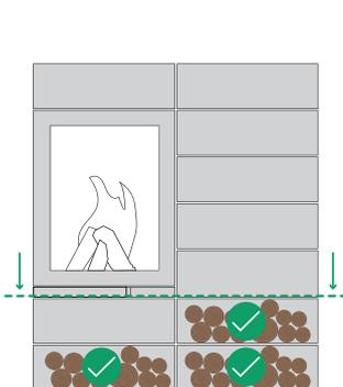
1. The element is located below or below/laterally from the firing chamber. Here, no significant heat transmission takes place. It is also possible to close this element by means of a flap.
