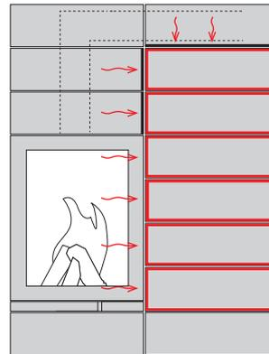
Technical box with radiation protection plate inserted
