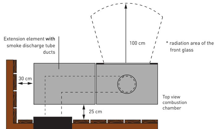
Extension elements, through which **smoke discharge tubes are fed** can be installed at a distance of at least 30 cm to **combustible elements** or walls (please observe the DIN of the smoke discharge tubes).
