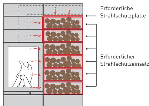
2. The element is mounted laterally at the firing chamber and is equipped with a special radiation protection insert against heat transmission. If further extension elements with smoke discharge tubes are provided above this element (for the storage of fuel), these must be equipped additionally with a radiation protection plate on the ground.
